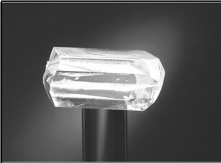
Fig 1: Gallium Phosphate crystal. Photograph from AVL List [2].
